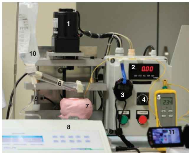
Fig. 1. Experimental set-up: 1, motor; 2, load cell display; 3, chronometer; 4, motor velocity regulator; 5, thermocouple with type K thermopar; 6, handpiece (Bienair ® ); 7, Labosil ® specimen stabilization; 8, Bienair ® implant motor; 9, magnetic sensor; 10, saline solution; 11, video camera.
