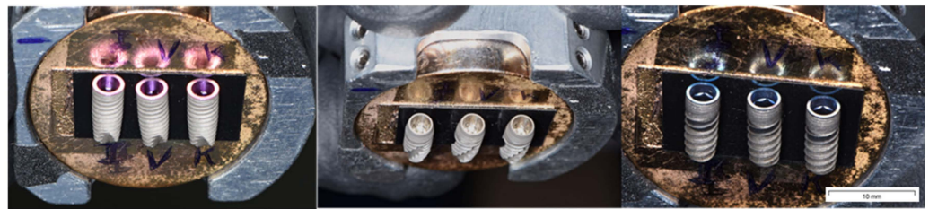
Figure 3. Implants placed in the sample holder of the SEM. Each implant brand was analyzed. The implants subjected to the highest torque presented visually detectable surface deformations at the level of the apical third.
