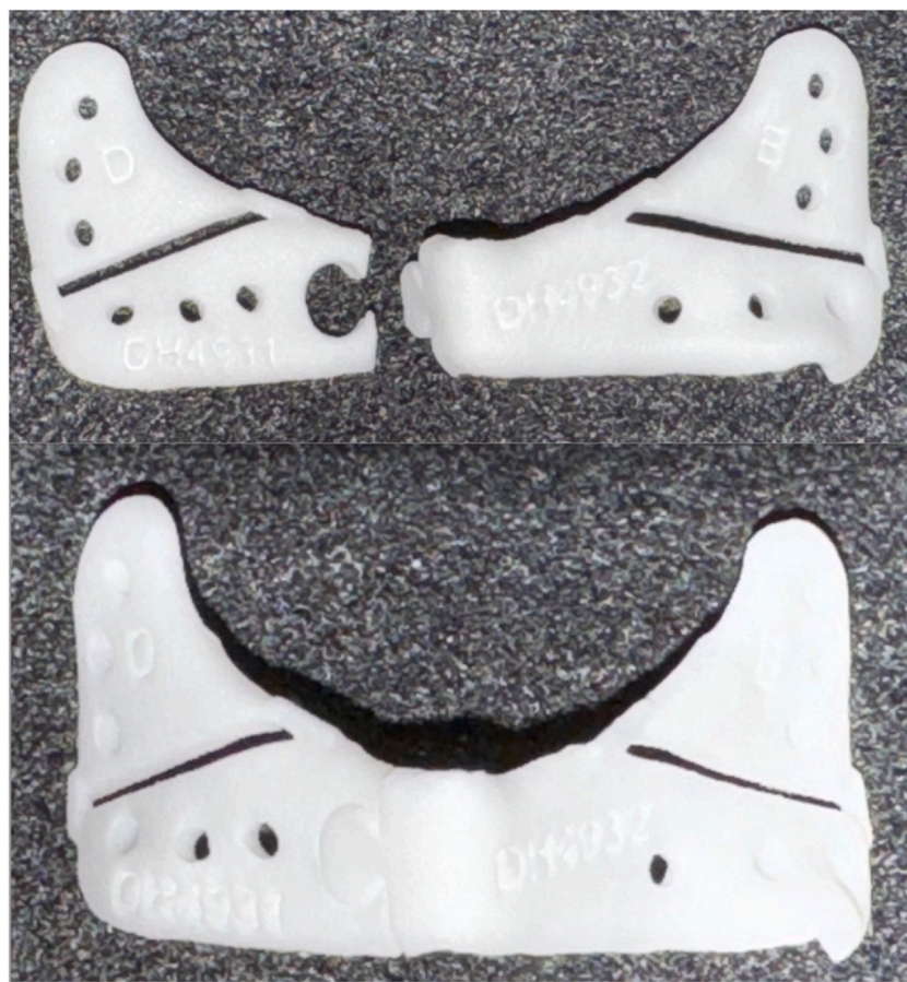
Fig. 3. Cutting and drilling guides printed using SLS technology.
