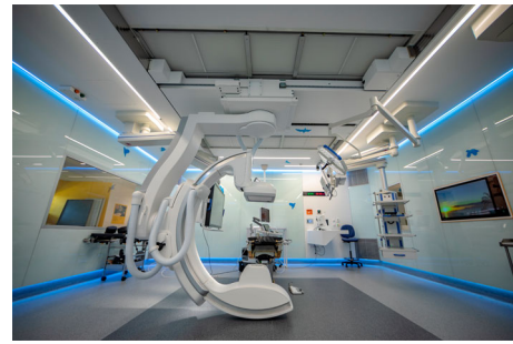
Fig. 1 Operating Room equipped with a low-dose C-arm ICBCT machine
